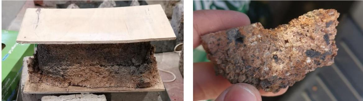
Figure 11 - Photos of bricks after crushing. New brick (L), Reclaimed brick (R)
