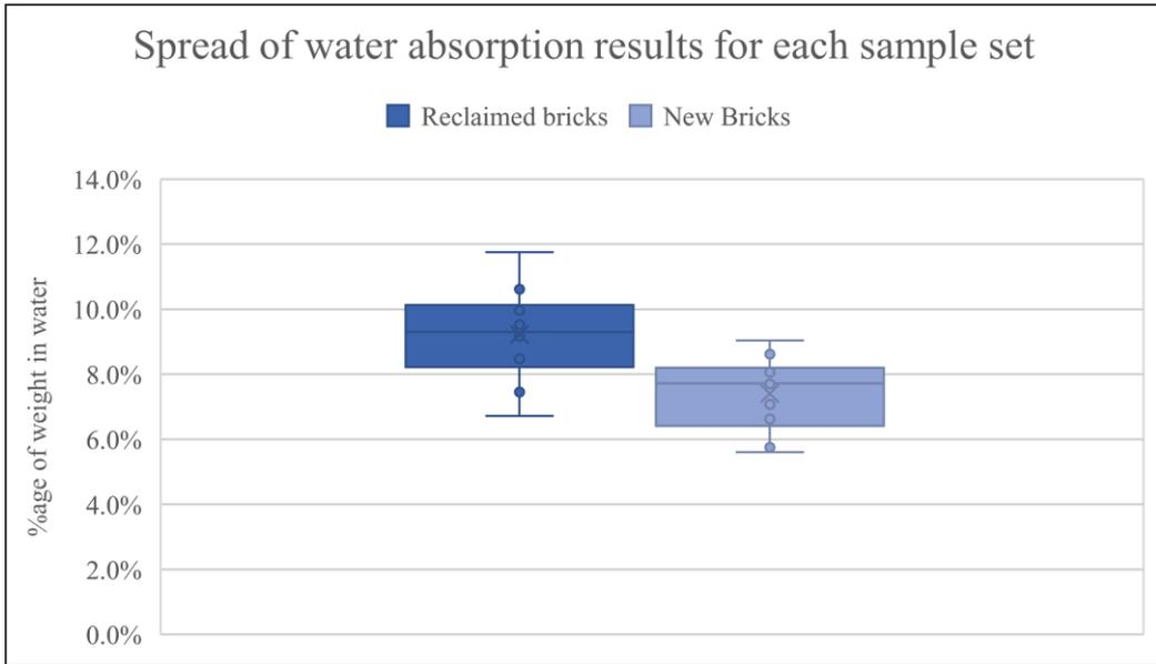
*Figure 7 - Box plot showing spread of water absorption results.*
