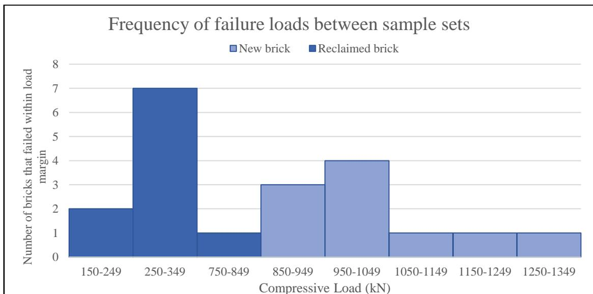
Figure 9 - Spread of compressive load at failure between sets.
