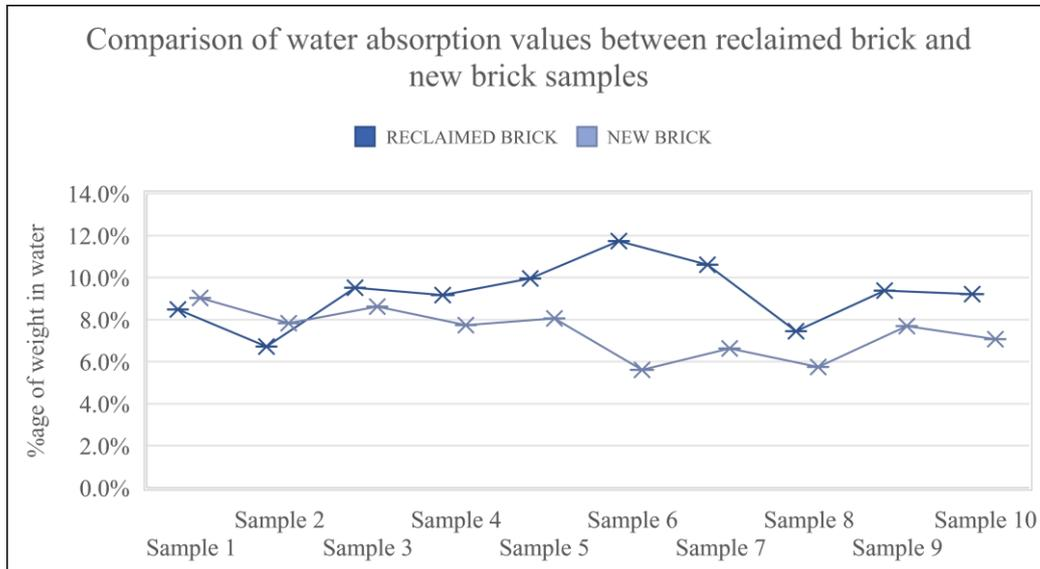
Figure 6 - Comparison of water absorption values of all samples
